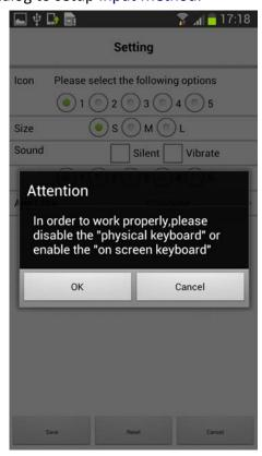
3. In order to make sure the on-screen keyboard will still function when operating with the micro USB barcode scanner (emulating an external keyboard), please switch off "Physical Keyboard" or switch on "On-screen Keyboard" if any. And then select your desired keyboard as input method.
