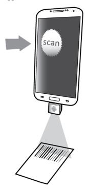
4. To scan a barcode, make sure the aiming beam crosses every bar and space of the barcode.
